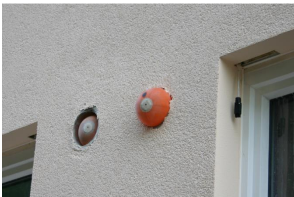
Temporary sealing of the outdoor air and exhaust air openings of the ventilation system during the measurement
